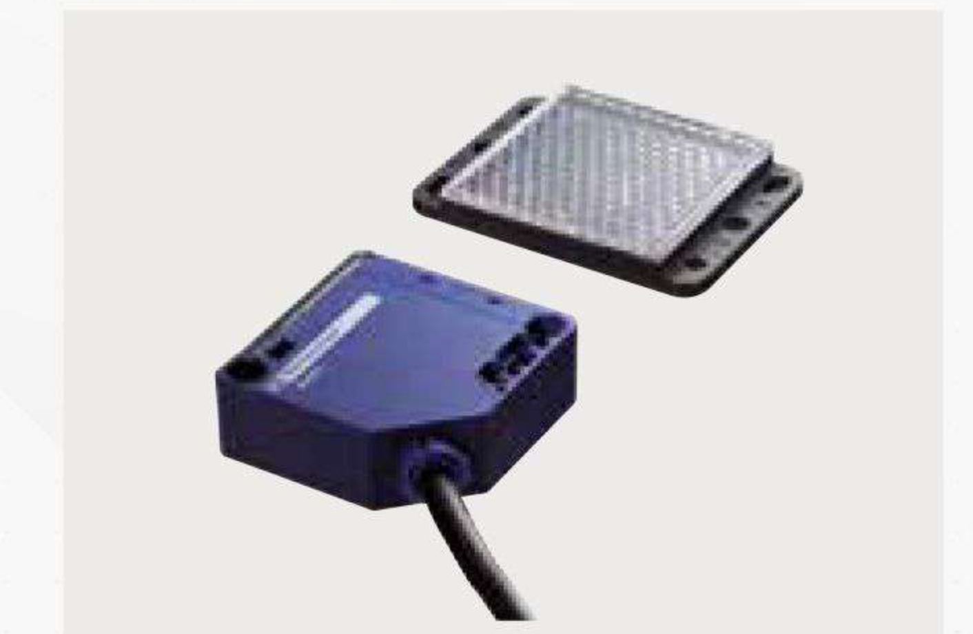
Extra 628 reflection light opto sensor 24-240 V AC, 12-240 V DC, IP 54 Range: 5 m Can only be used as a pulse generator
